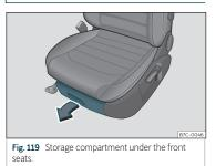
*Opening*: Press the tab on the drawer handle and take the drawer out.
