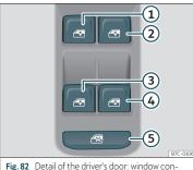
Fig. 82 Detail of the driver's door: window controls.
