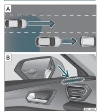
Fig. 162 Schematic representation: A Passing situation with traffic behind the vehicle. I Indication of the lane departure warning in the control lamp on the left side.
