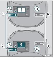
Fig. 42 Diagram of connections for vehicles with Start-Stop system.
