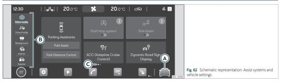
Press  $\square \gg$  Fig. 62 (a), or Vehicle settings in the main menu to open the assistants and vehicle settings menu. Next, clicking on any of the menus located in the left area (b), displays the settings menu or the selected assist systems on the display.
