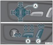
Fig. 96 Driver's seat: electric seat settings.
