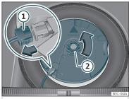
Fig. 198 In the luggage compartment: remove the subwoofer.
