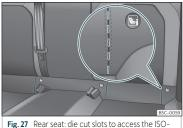
Fig. 27 Rear seat: die cut slots to access the ISO-FIX / iSize securing rings.
