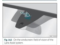
Depending on the equipment, the vehicle may be fitted with a front camera on the front windscreen»» Fig. 142. This camera detects lane boundaries (lines) to provide support for the following functions:
