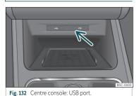
Depending on the equipment and the country, the vehicle may also have USB connections **exclusively for charging or as a power socket**.
