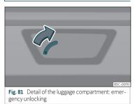
The rear lid can be unlocked from inside in the event of an emergency (e.g. no battery).
