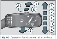
Fig. 90 Operating the windscreen wiper and rea wiper.
