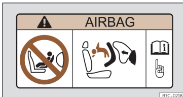
Fig. 23 Airbag sticker: on the passenger's sun visor
