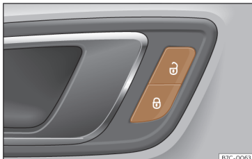
Fig. 70 Driver's door: central locking switch.
