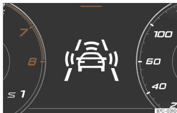
Fig. 151 On the instrument panel display: advance warning indications.
