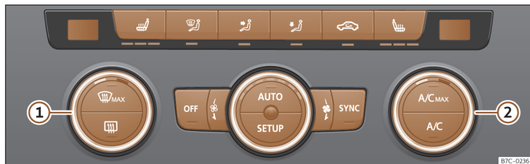
Fig. 124 In the centre console: Climatronic controls.
