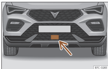
Fig. 143 On the front bumper: radar sensors.
