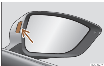
Fig. 164 Control lamp of the lane departure warning.
