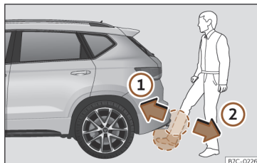
Fig. 80 Rear lid with sensor-controlled opening (Easy Open).
