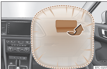
Fig. 14 Front passenger airbag located in dash panel.
