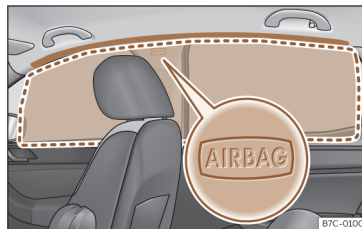
Fig. 21 Location of head-protection airbags.
