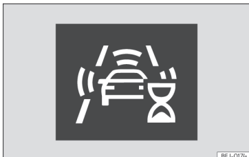
Fig. 153 On the instrument panel display: initial system self-calibration indication.
