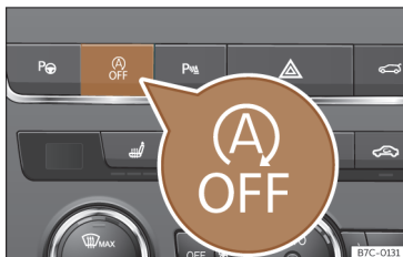
Fig. 136 Centre console: Start-stop system button.
