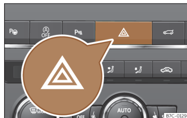
Fig. 90 Dash panel: hazard warning lights switch
