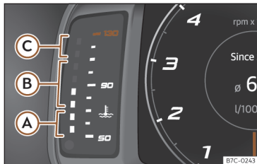
Fig. 55 Engine coolant temperature indicator.
