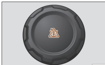
Fig. 200 Engine compartment: coolant expansion tank cap.
