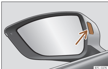
Fig. 163 Control lamp of the lane departure warning.
