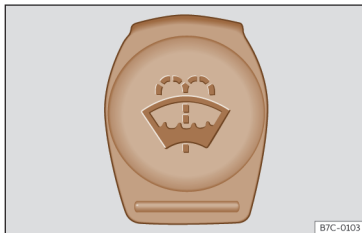
Fig. 202 In the engine compartment: window washer tank cap.
