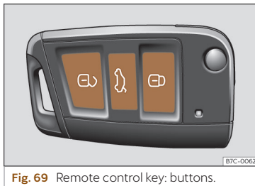
Fig. 69 Remote control key: buttons.
