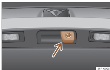
Fig. 155 In the rear lid handle: location of the reverse assist camera.
